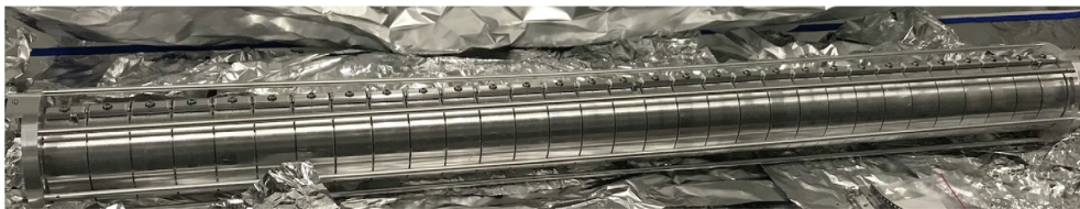
Fig. 3. The electron repeller consisting of 31 electrodes.
