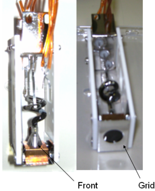
Figure 6.5: Photograph of the channeltron detector showing the energy selection grid, which was grounded during moderator growth.
